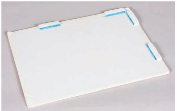
Figure 11-4 Foam-core board paper prototype easel with “stops” to align the interaction sheets.
