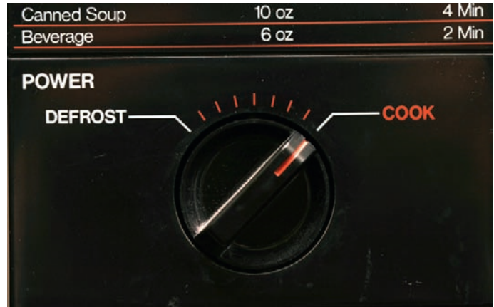
Figure 20-5 Useless dial marks between power settings on a microwave.
