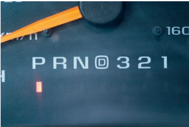
Figure 22-55 Typical automatic transmission shifting pattern.
